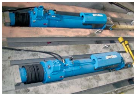
Fig. 13: 1500 kN/1300 mm stroke synchronized detensioning cylinders with automatically tightened adjusting ring nut
