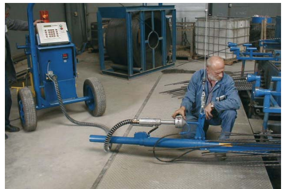
160 kN/500 mm stroke for 1/2" strand with TENSACONTROL unit used for stressing roof trusses
