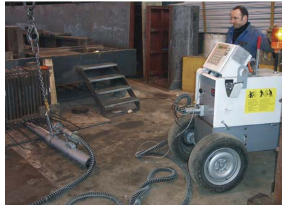
300 kN/400 mm stroke for 0.6" strand with TENSACONTROL unit on stressing bridge beams
